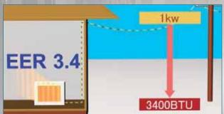
An electric heater converts electricity directly to heat, and if we assume that the heat loss is zero, the output from one kilowatt input is one kilowatt or 3,400 BTU and the EER is 3.4.
